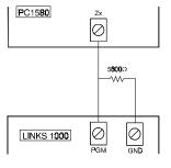
The LINKS Supervisory zone must be wired according to the accompanying diagram.
